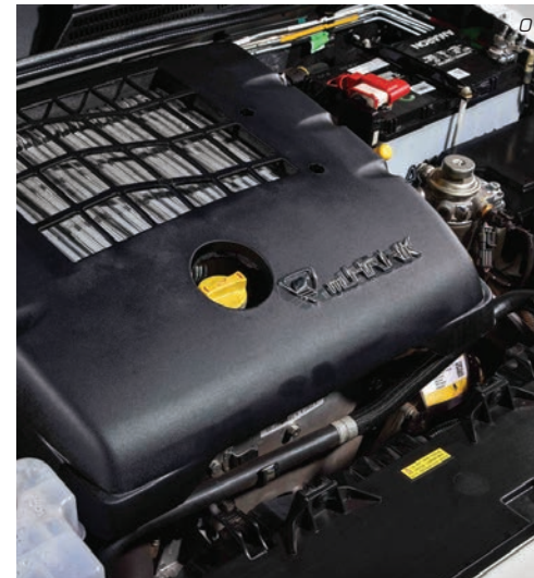
01 - Mahindra's legendary 2.2l mHawk turbo-diesel engine with new 5-speed manual transmission.
